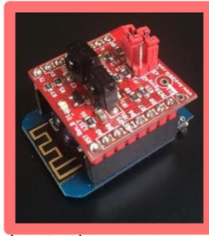
A getting started guide is also provided, with every order. The A.IR Shield ESP8266/ESP32 TRx is also pin compatible with the ESP32 Mini D1. Firmware & AnalysIR support for both the ESP8266 and ESP32 Mini D1 is available now & provided with each purchase.
