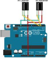
from the list on the right. You will also require an infrared receiver and optionally an IR Learner. (Recommended IR Receiver: TSSP4038, TSSP58038 or TSOP34438; and the optional IR Learner: TSMP58000). Of course, you can use your existing IR receiver. LEARNIR and USB IR Toy do not require any additional IR components or configurations.
